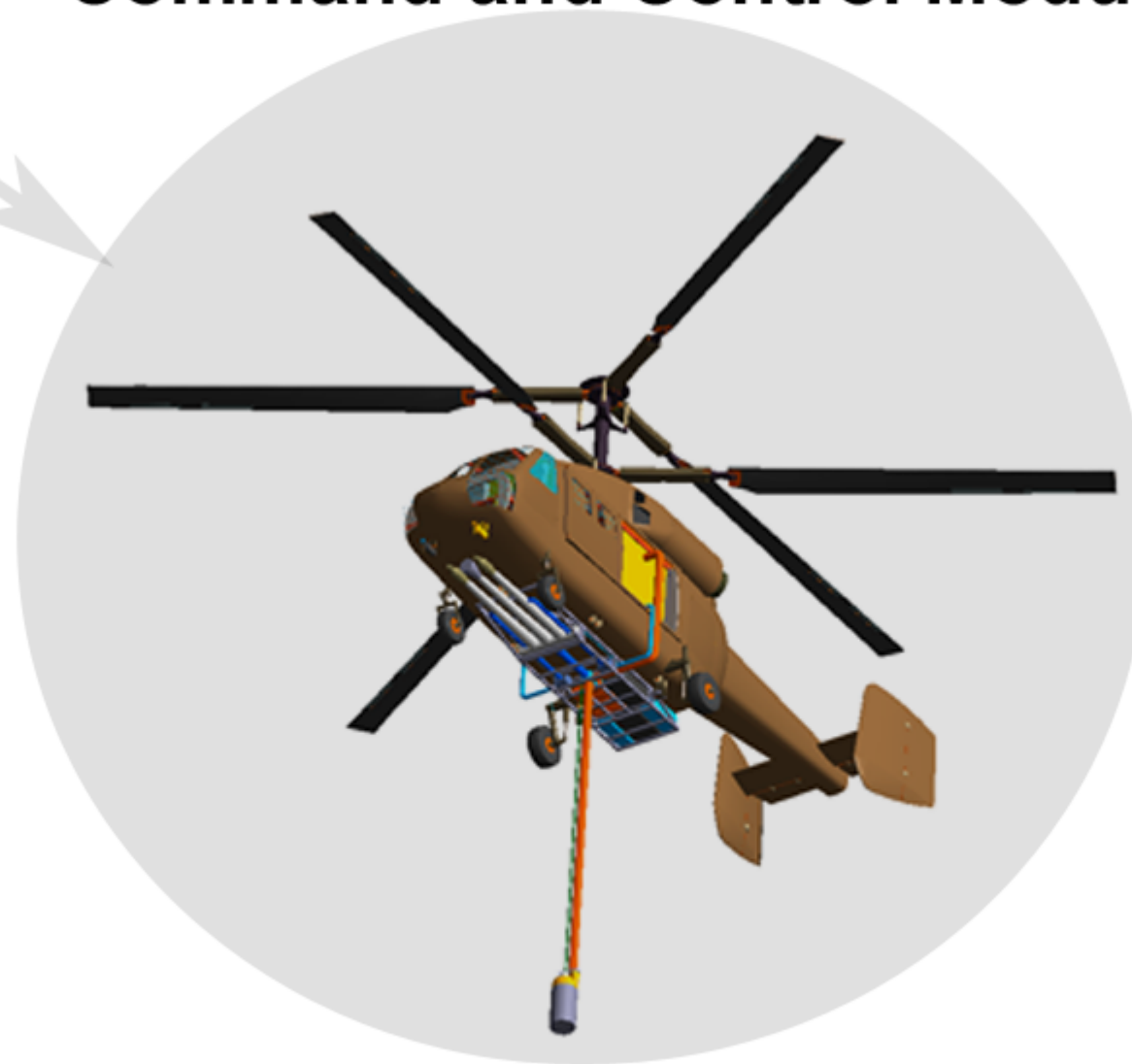
Self Contained Firefighting Module
